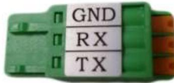
To connect a serial device, map the pins as below:
