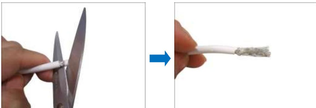
5. Twist the braid or tinned copper wires together and remove the foil coating.
