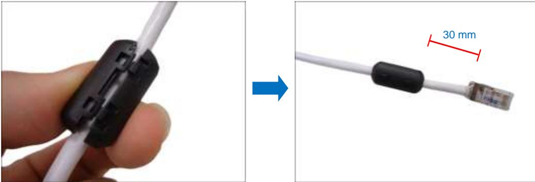
**NOTE:** The ferrite core is used to suppress electromagnetic interference (EMI) from the camera that may affect other devices, as well as prevent the EMI from other electronic devices to affect the performance of the camera.
