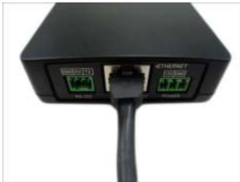
2. Connect the other end to a switch or injector. Then, connect the switch or injector to a network or PC and a power source. See Power-over-Ethernet (PoE) example connection diagram below.
