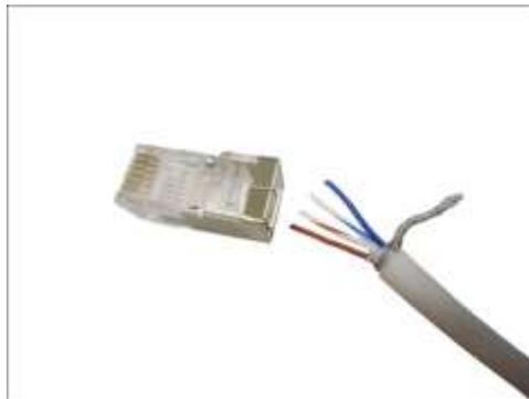
8. Place the connector into the crimping tool, and cinch down to secure the RJ-12 connector to the cable.
