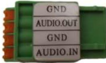
To connect audio input / output devices, map the pins to one of the pin combinations below:
