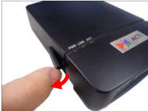
2. Insert the memory card with the metal contacts facing down the main unit.
