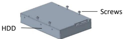
2. Insert the screws into the disk and tighten the screws halfway.
