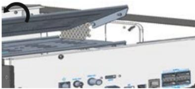
3. Secure the disks on the mounting plate. Fix the screws according to the figure below. Avoid damaging the disk in the process.
