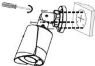
8. Point the camera at your preferred surveillance target, and then tighten the locknut.
