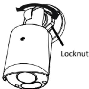
7. Attach the camera to the surface.
