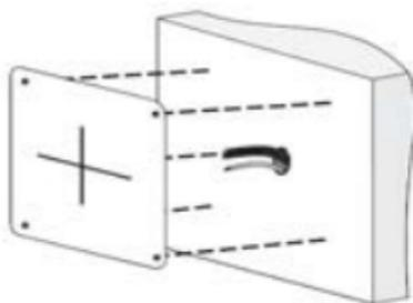
3. Drill  $\frac{1}{4}$ " holes  $1\frac{1}{4}$ " deep into the surface for the mounting screws. If cables are routed beneath the surface, drill a hole for the cables to pass through.
