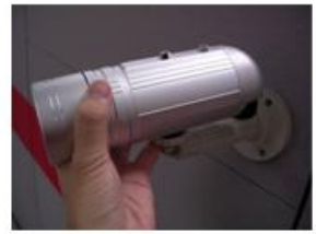
6. Remove the camera cover
